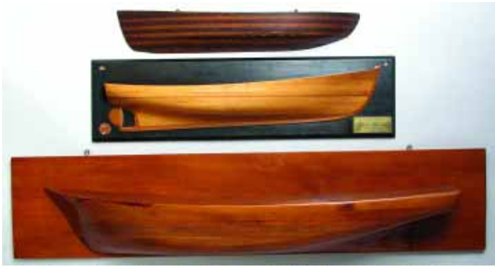
300. SHIPWRIGHT'S HALF HULL MODEL OF A PINKY, 2 nd half of the 19 th Century, built in lifts. Height 5 in. Length 32 ¼ in.
