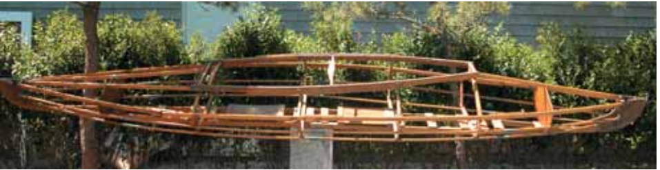
320. SCARCE FOLDING KAYAK FRAME, circa 1910-20, folds and disassembles to backpack size and enables wilderness kayaking after the skin is applied. Length 13'1"
